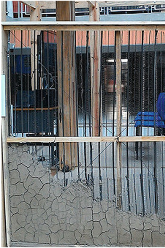
Fig. 7 Panel 3, steel mesh core with two earthen mixtures layers
